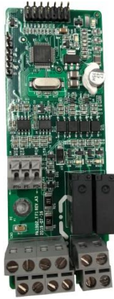
IO expansion card 2 EC-IO502-00
