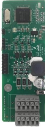
Simplified incremental PG card EC-PG507-12
