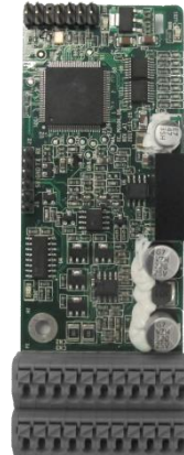
Resolver PG card EC-PG504-00
