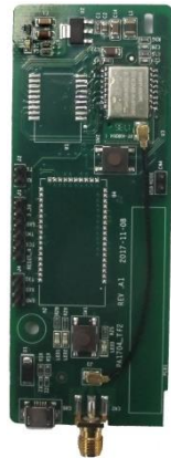
Bluetooth/WIFI communication card EC-TX501/502
