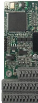
UVW incremental PG card EC-PG503-05
