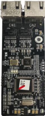
Ethernet/IP communication card EC-TX510/ Modbus TCP communication card EC-TX515
